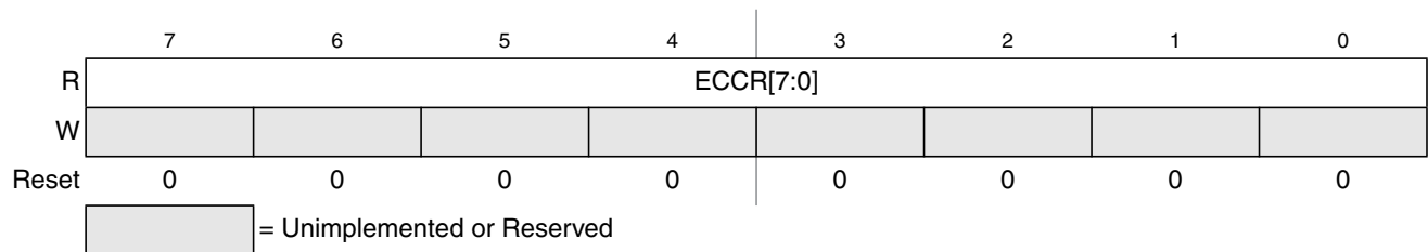
Figure 28-21. Flash ECC Error Results Low Register (FECCRLO)
