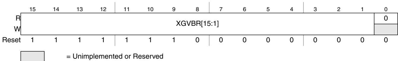
Figure 10-9. XGATE Vector Base Address Register (XGVBR)
