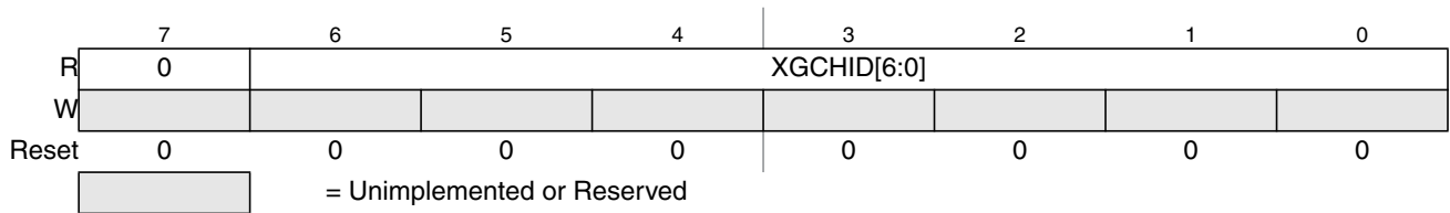
Figure 10-4. XGATE Channel ID Register (XGCHID)
